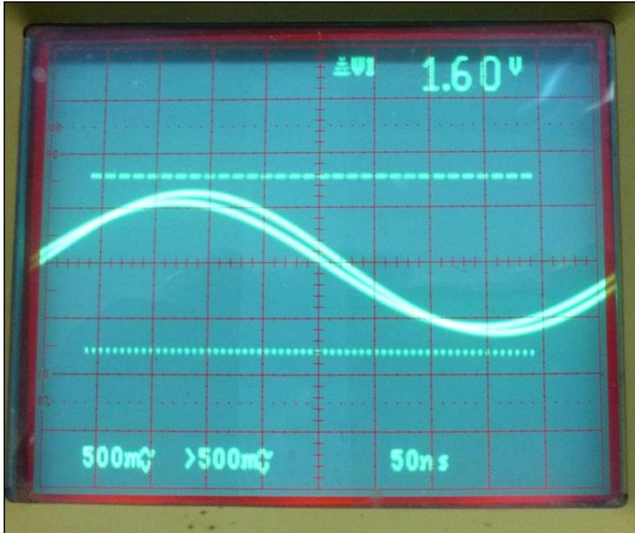
**Soft Clipping**-note the output signal has been limited and it is not a square wave. It is rounded. The soft clipping reduces the harmonics and IMD products of a hard diode clip circuit. The **input level** is about 10-11 dBm which is the threshold many modern day receivers for no damage. Some transceivers can take 13-15 dBm.
