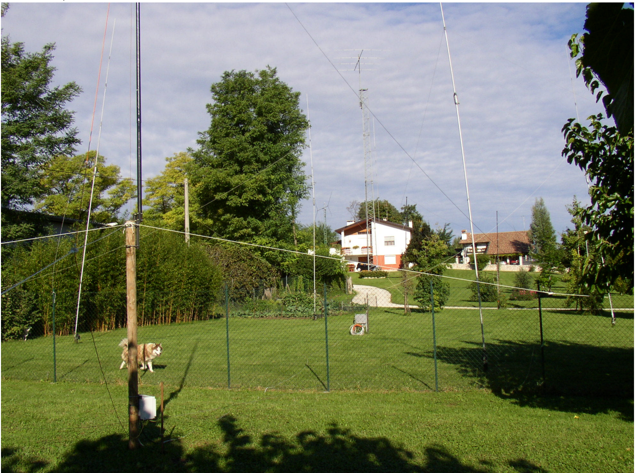
Fig.1 - IV3PRK 160 m. antennas: in front the K9AY loop, than the 4-squareRx mini-array, the southern group of Pennants, the shunt-fed tower and, on the back, the rotatable Flag
