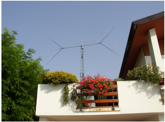
Fig.2: The W7IUV rotatable Flag at IV3PRK
