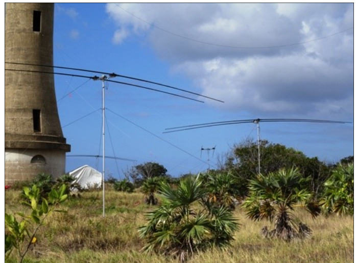
Four 2-element SteppIR beams on 7-meter masts.
