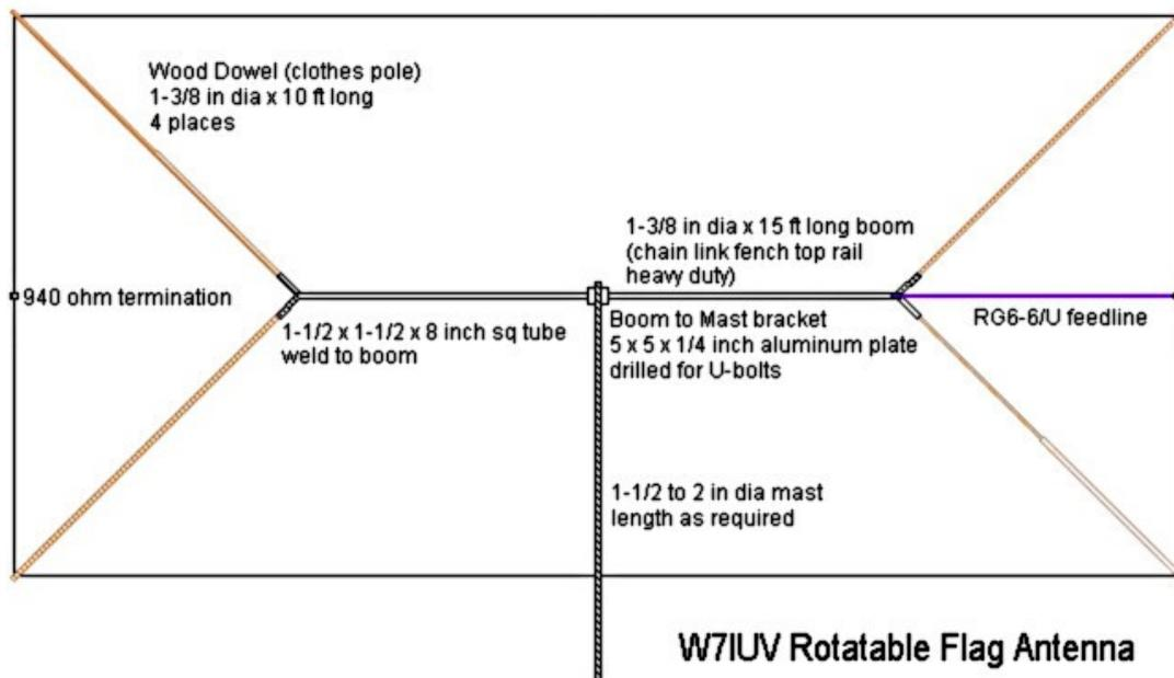
If welding is not your thing, consider making a spreader mounting plate from a square piece of aluminum about 12x12x1/4 inch. Drill for U-bolts in appropriate places.
