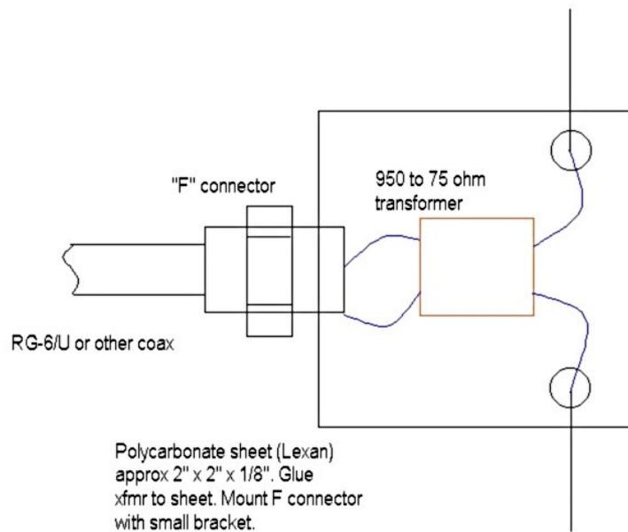
The transformer is just glued on. Mount a TV type F connector on a small bracket. F connectors are real cheap and great when using RG-59/U or RG-6/U 75 ohm coax. If you need to weatherproof it, paint the whole business with PVC pipe cement, several coats, and spray with black Krylon paint. The insulator for the termination resistor is made the same way.
