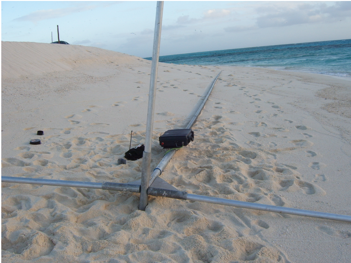
18 meter SpiderPole with aluminum base before erection. Note that the fourth leg of the base has not been inserted yet.
