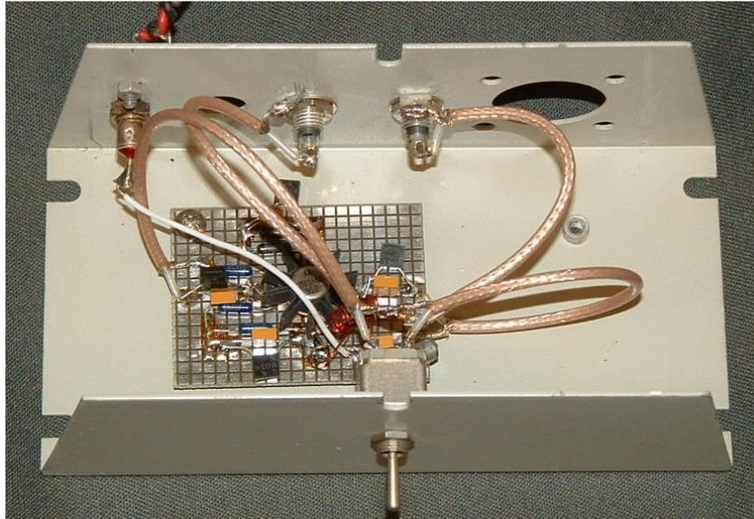
The photo above shows a preamp assembled on “checkerboard” and installed in a small salvaged chassis. The toggle switch is used to bypass the preamp. This unit was used for some VLF SWL'ing.
