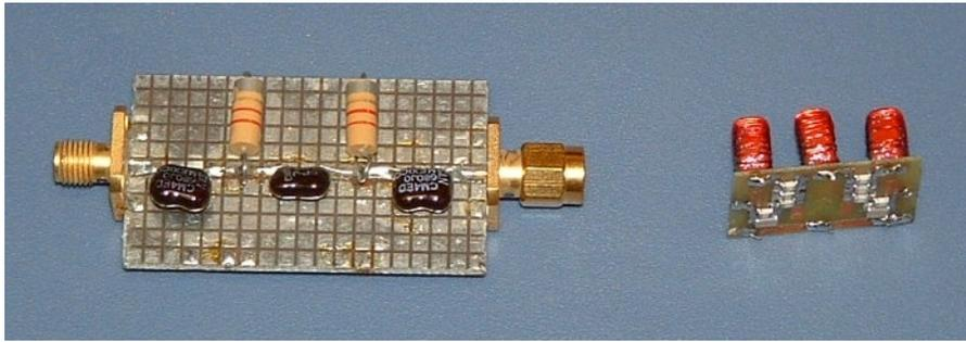
The filter should be in a shielded enclosure. It can be in the same box as the preamp. Separate modules will allow some extra versatility and if connectors are used, will allow changing filter designs easily.
