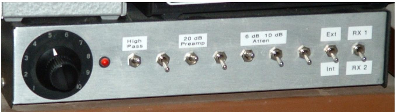
The above photo shows the preamp system I have used daily on the low bands for the last 15 years or so. It has a rotary switch that allows selection of various RX antennas. There is a high pass filter and attenuators built in which can be inserted or bypassed with the small toggle switches. The toggles on the right end allow selection of different radios and cable routing. More info on this box will be given later. Some of the labels are missing in this photo.
