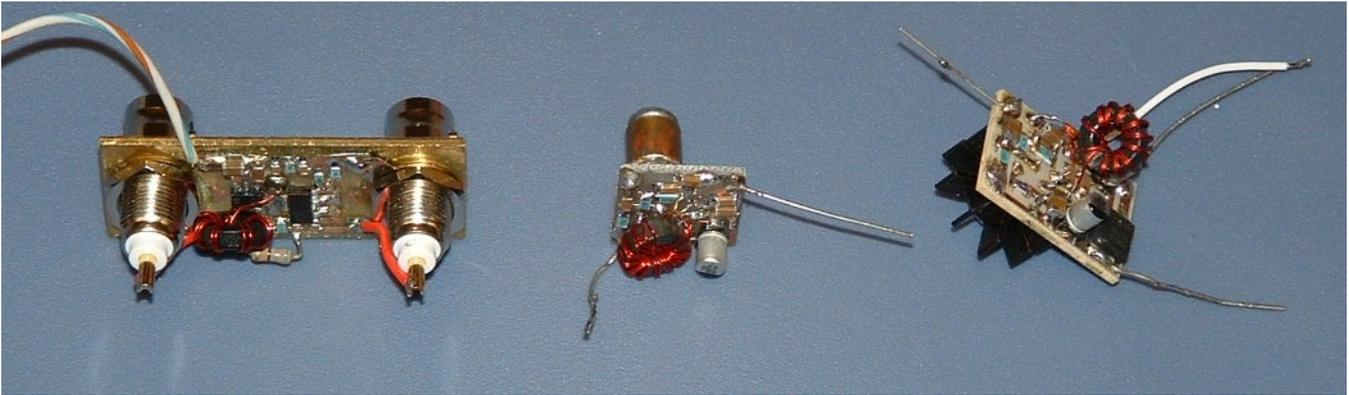
The above photo shows a few of the surface mount assemblies produced by W4EDS (SK). Ed submitted them to me for evaluation. They performed superbly. Note the size of these modules. The core diameter is 3/8 inch. Variations using 2N5109 as well as the DCP68 are shown. The wires hanging off the edges are mine and used for testing on the bench, usually input, output, Vcc, and ground.
