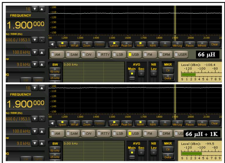
with a shield around only the inductor grounded to the ground plane of the amp PC board, and with a second shield enclosing the amp and shielded inductor.
