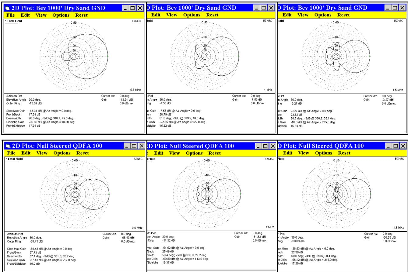
Much shorter (~150 total linear feet) versions of this fixed null steered QDFA with greater than 13 RDF can be designed for higher frequencies, such as for the 160 through 40 meter ham bands (and all frequencies in between).
