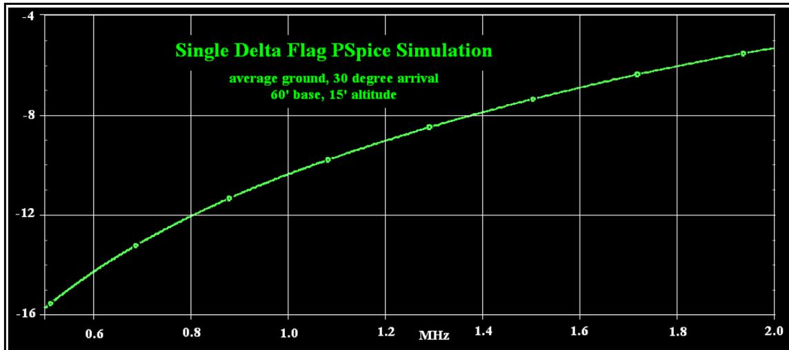
The single delta flag simulation above is for reference. Below is a single active delta flag simulation.
