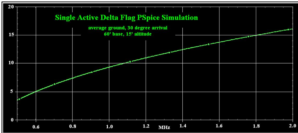
As can be seen, activating a delta flag antenna element with a FET follower is equivalent to adding a 20 dB gain 0 dB noise figure preamplifier. This was verified with repeated tests at my location just outside Ruston, LA in the summer and fall of 2011 and at Quoddy Head in November 2011 with a dual active delta flag array.
